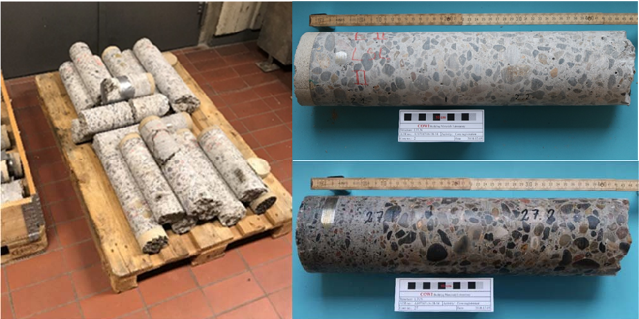
Figure 6.1-2 Cores extracted from wall (cores without fire protection) and roof (cores with fire proofing).
