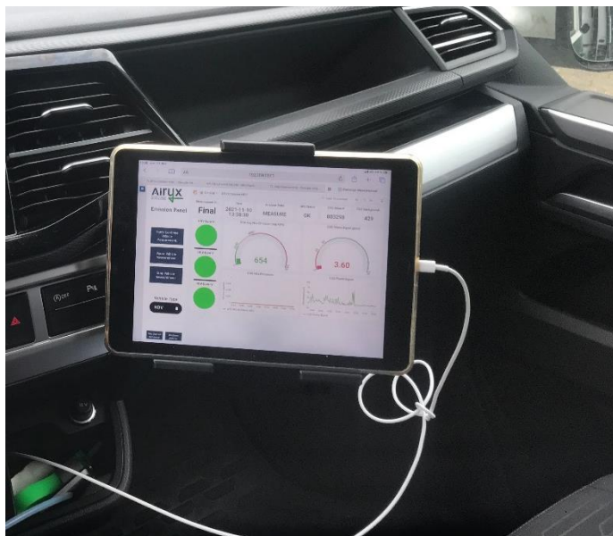
Figure 2: The tablet that is used to show the plume chasing measurement during the drive.
