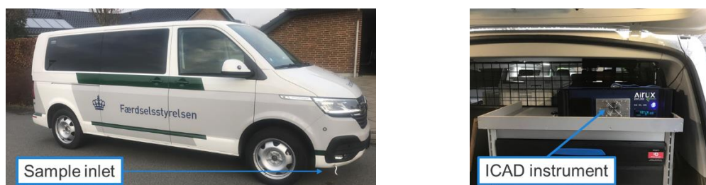
Figure 1: The vehicle with the plume chasing equipment mounted. The image to the left shows the sample inlet. There are two sample inlets one on each side in the front of the car. The image to the right shows the analyzer mounted in the back of the car.
