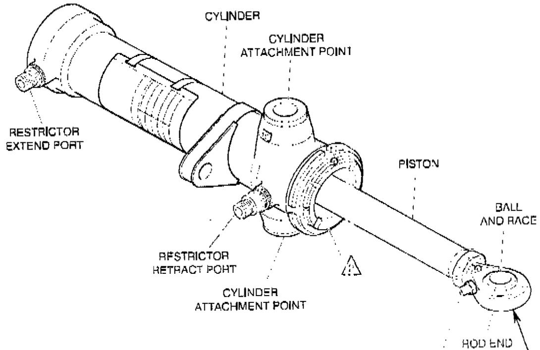
Remove the rod end of the retraction actuator assembly in accordance with SCR 086-07 rev. NC
