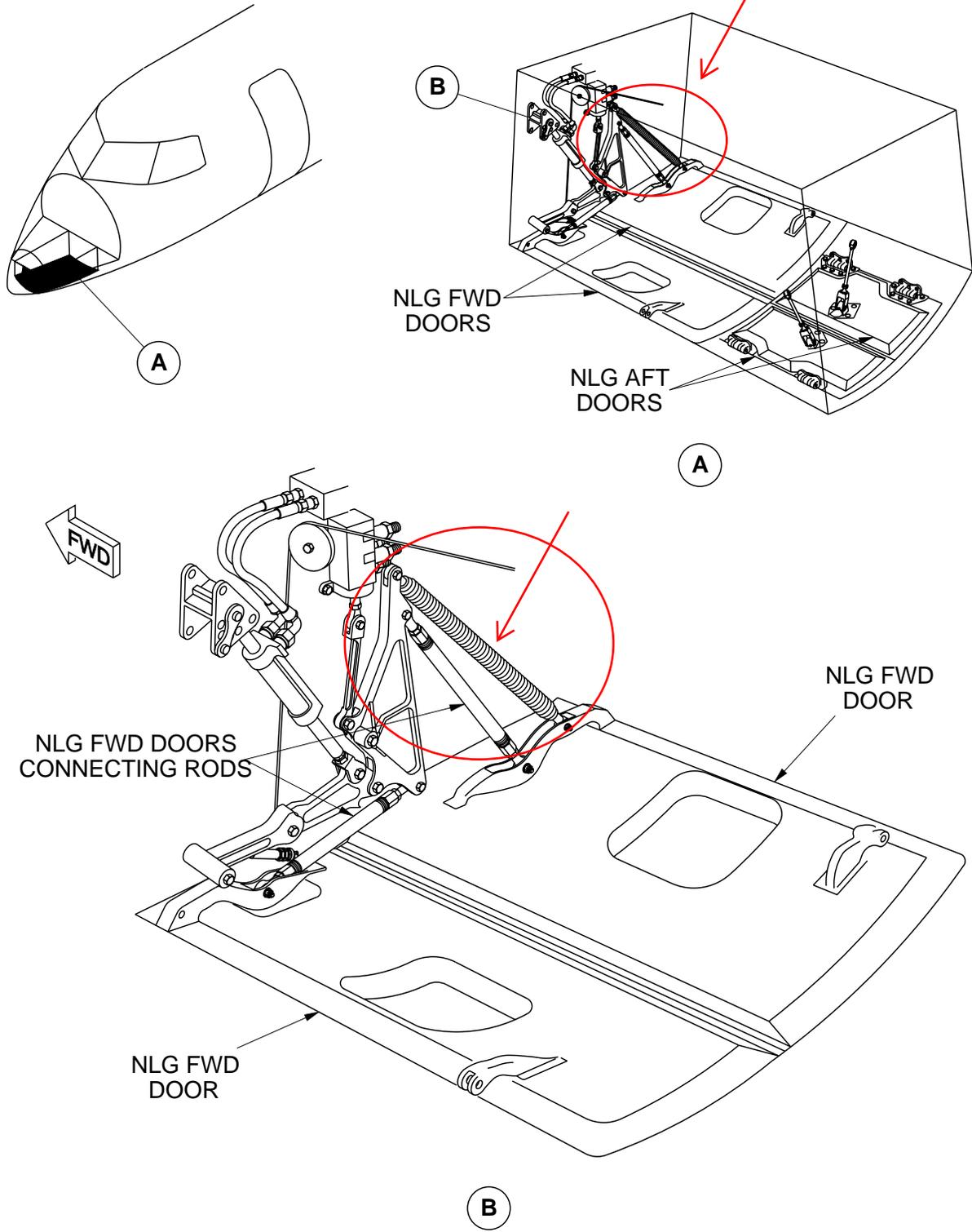
Nose Landing Gear Doors – Component Location
