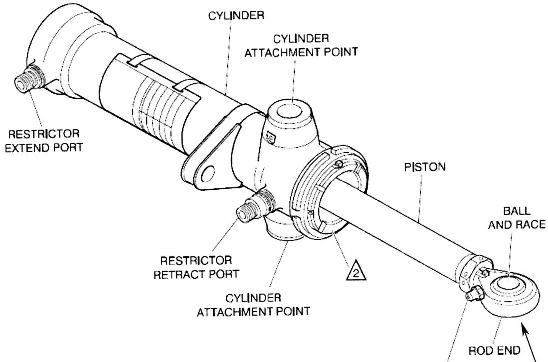
Remove the rod end of the retraction actuator assembly in accordance with SCR 086-07 rev. D
