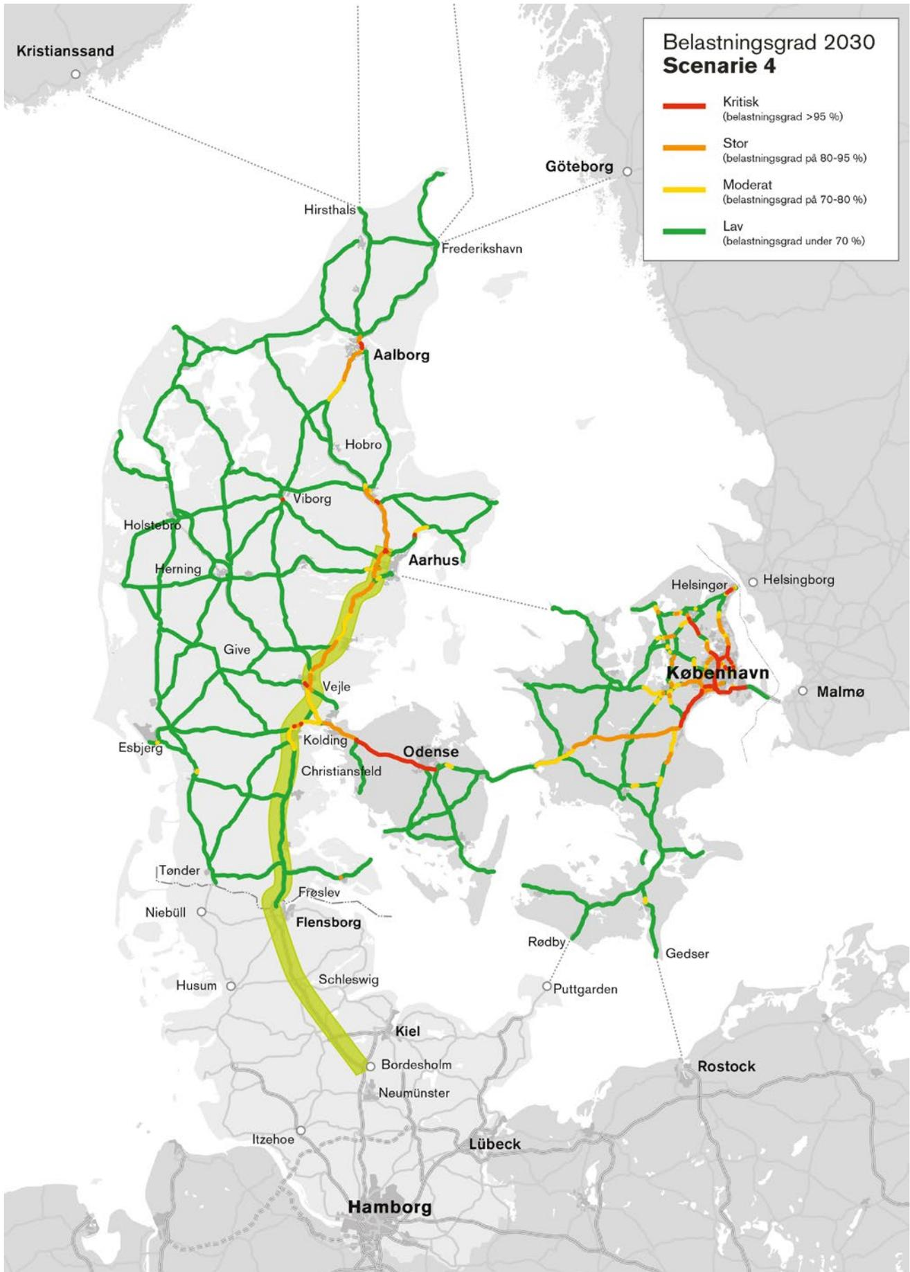
Map 4.10: Traffic load ratios on the main road network in 2030 if the E45/A7 is partially expanded.
